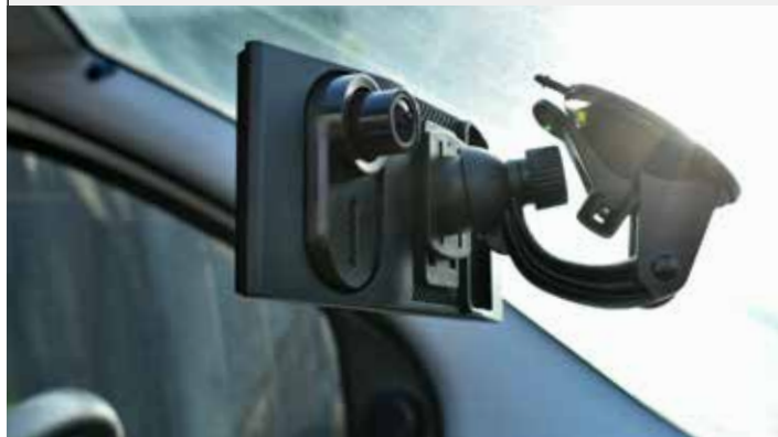
WINDSCREEN INSTALLATION WITH INCLUDED ADJUSTABLE DEDICATED MOUNT
